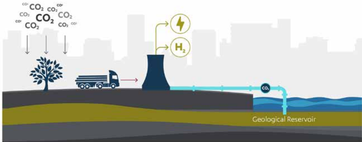
Figure 1.4: The bioenergy with carbon capture and storage process
