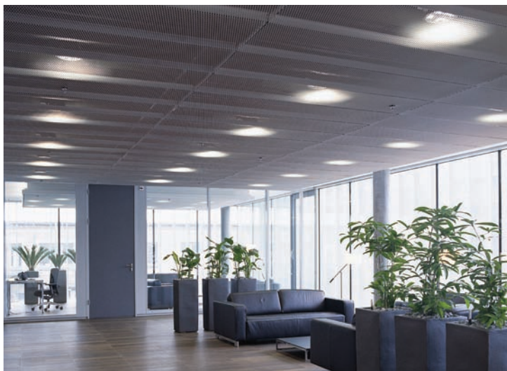
Armstrong's OP19 metal ceiling systems have a 30% recycled content
