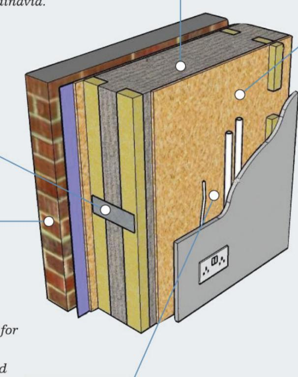
Airtightness. The oriented strand board is used as the primary air seal for the walls. The panels are designed with lock joints and factory fitted compressible foam seals at the head and foot of the panels which form a seal between the panel and the sole plate. Vertical joints are taped. This approach does away with the need for a separate air membrane and should achieve an air permeability of  $3m^3/h/m^2$ .
