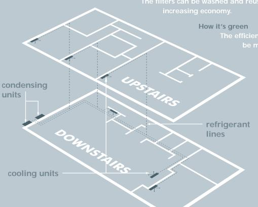
(CoP). This particular wall-mounted system boasts a CoP rating of 3, meaning that for one unit of electricity used, three units of cooling power are produced. This equates to 300%, and is three times as efficient as standard air conditioning units which commonly have a CoP of only 1.
