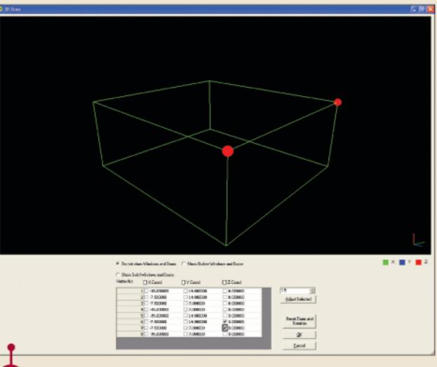
The geometry for each zone can then be adapted in a 3D editor. This can be used to perform elaborate editing and the generation of complex geometries. Finally, the whole building can be viewed within a 3D viewer to ensure that it looks correct. Images can also be taken from this viewer for presentation in reports.
