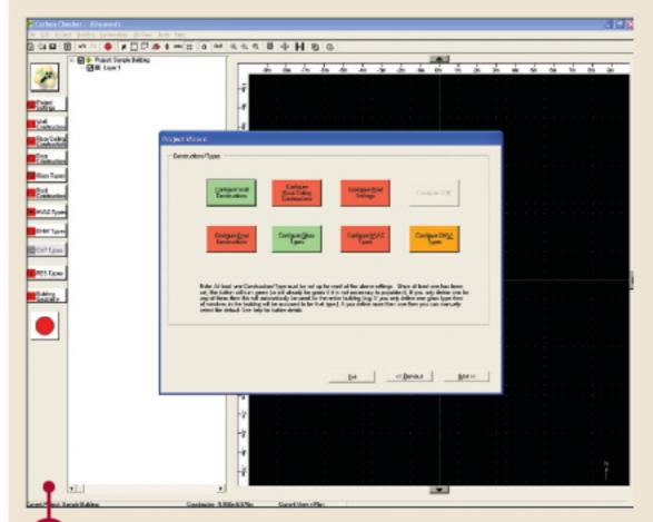
1 To create a project, first-timers are encouraged to use the project wizard, which guides you through the initial settings (eg project details; construction; glazing, HVAC, DHW and CHP settings etc). It⊠s a simple way to enter the minimum settings required for a valid SBEM
