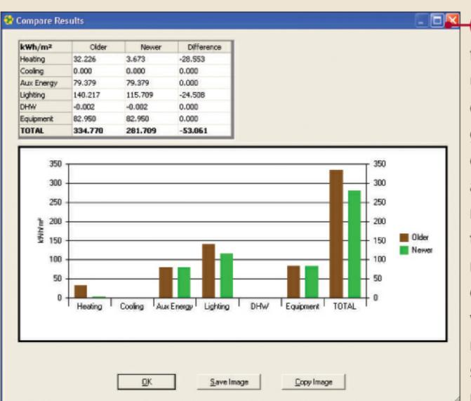
fails to comply, the user must change either the building geometry or services. Any number of alterations can be made and run through, and all results are presented in the output viewer so that the most technically feasible and economic route to compliance
