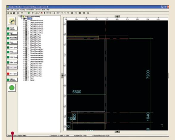
3 A DXF file (easily created in CAD packages eg AutoCAD) can be imported into Carbon Checker to allow tracing over for quick creation
