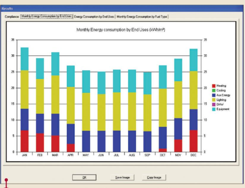
When all the required data is available the SBEM button turns green and the calculation can be performed. The BER and TER are calculated together with the official Part L2 compliance checking module, BRUKL. This reveals whether the building has passed the compliance checks and also provides detailed energy performance reports.
