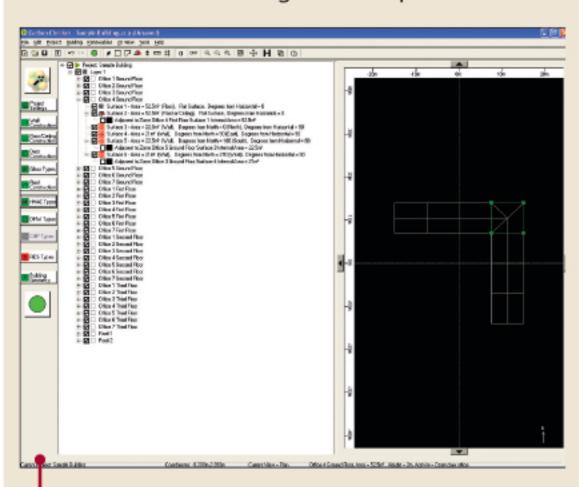
4 Once the building zones are identified by space type and activity, the geometry can be defined. A 2D design interface is used initially to create the building model. The model above has been built up by creating a zone and then copying and pasting to create identical office
