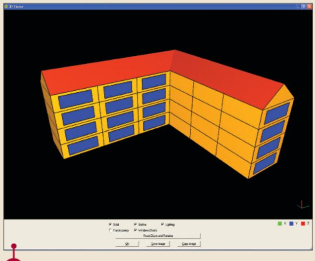
The next step is to add windows and doors to the zones. To do this, a simple 2D surface editor is provided. To help the user assess the impact of different glazing options, the size of windows can be increased or decreased globally for each orientation, eg 50% glazing can be added to all southern aspect walls.
