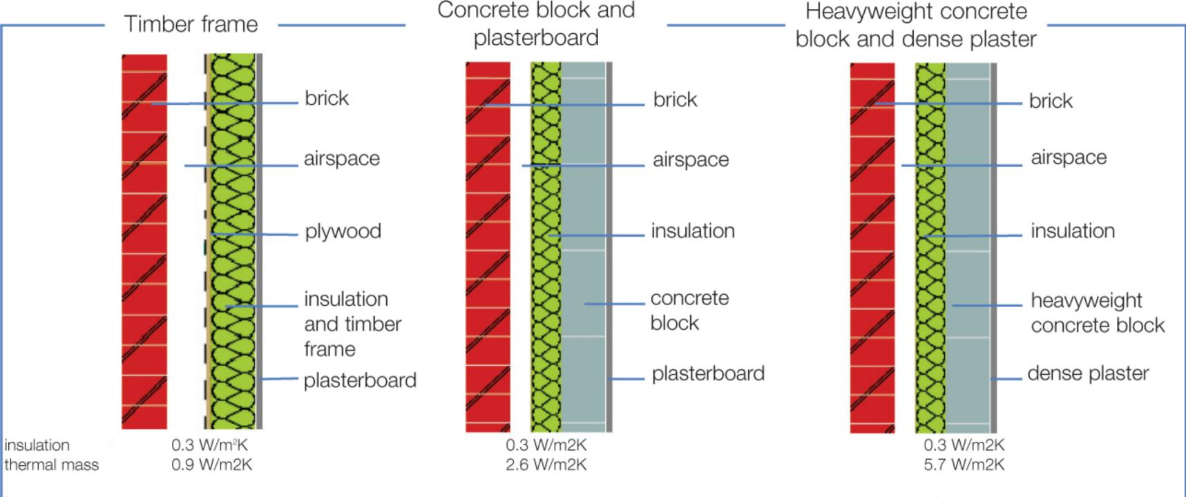
(insulation relates to the transfer of energy through the wall; thermal mass relates to the storage of energy in the inner skin of the wall)
